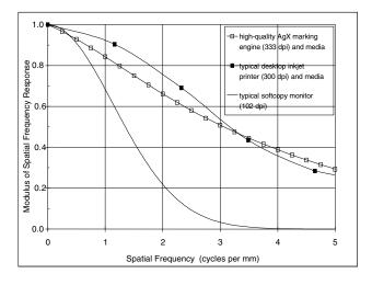
Figure 1. The MTFs of three device-media combinations.
