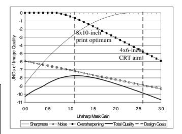
Figure 3. The effect of spatial filter gain level on the quality attributes of a particular 3.1-mega-pixel DSC capture written to 8 x 10-inch reflection media at 333-dpi.
