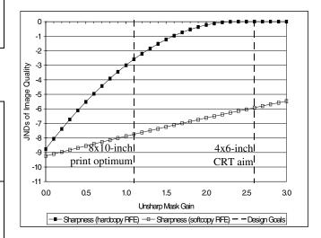
Figure 4. The effect of spatial filter gain level on the perceived sharpness of a particular 3.1-mega-pixel DSC capture written to 8 x 10-inch reflection media at 333-dpi and displayed at 4 x 6-inch size on an 102-dpi CRT monitor.
